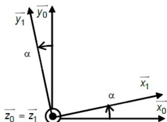
$$\begin{aligned} \vec{x}_1 &= \cos \alpha \cdot \vec{x}_0 + \sin \alpha \cdot \vec{y}_0 & \vec{x}_0 &= \cos \alpha \cdot \vec{x}_1 - \sin \alpha \cdot \vec{y}_1 \\ \vec{y}_1 &= -\sin \alpha \cdot \vec{x}_0 + \cos \alpha \cdot \vec{y}_0 & \vec{y}_0 &= \sin \alpha \cdot \vec{x}_1 + \cos \alpha \cdot \vec{y}_1 \end{aligned}$$
